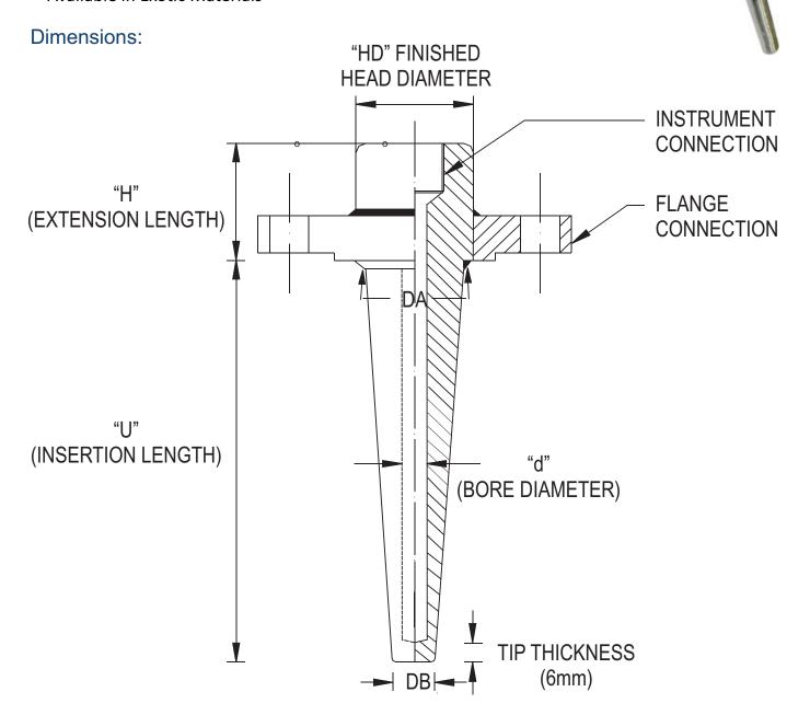
All Dimensions are in mm, Drawings are not to scale
